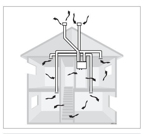
DO NOT SWITCH OFF THE UNIT! The system is designed to run continuously. If the unit is switched off indoor pollutant and moisture levels are likely to increase.
